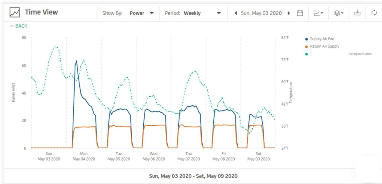
*Site Watch Application* – Using Time View and downloaded .CSV data, SiteWatch worked with the channel partner and equipment manufacturer to identify the VFD programming issue and assisted with real-time verification the drive was operating as intended. Ongoing measurement in the post-installation period was used to secure utility incentives.
