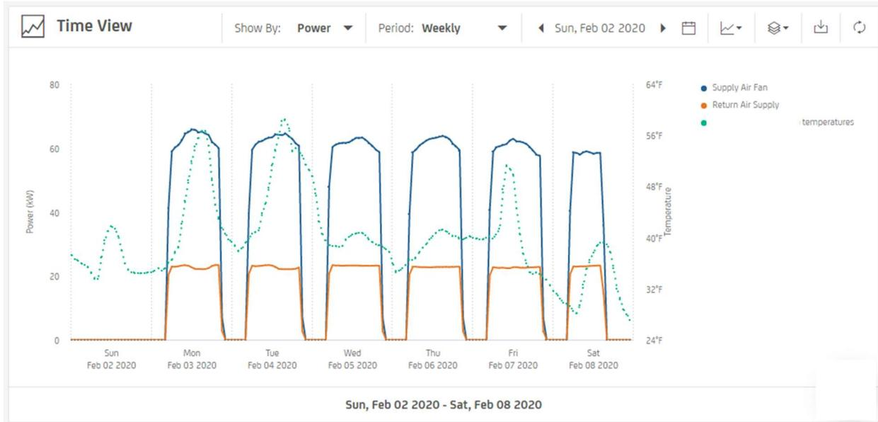
*Site Watch Application* – The channel partner identified excessive kW during operating periods when the variable speed device should have allowed motors to unload. Energy use during operating periods was higher than in the baseline.
