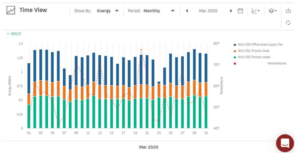
**Site Watch Application** – Site personnel can interact with SiteWatch to calculate ROI on proposed upgrades to existing constant volume air handling units while also enabling alarms on process area fans for over and under amp conditions.
