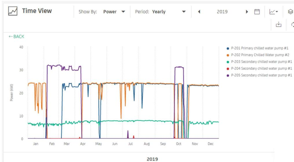
**Site Watch Application –** Site Watch reviewed pump data through time view to identify usage patterns and relationships between how pumps operate. The recommendations based on this data review would be to alarm low amps on primary chilled water pumps to ensure a backup pump is enabled quickly.
